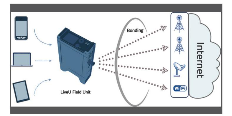
LiveU's DataBridge is a powerful mobile hotspot that offers resilient mobile broadband connectivity for multiple devices in any location, by bonding together existing multiple cellular and other data connections.
